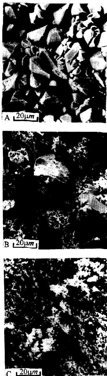
Fig. 3. (A) SEM of the active mass for a passivated negative plate before the sweep of Fig. 1(A). (B) After undergoing one cycle of Fig. 1(A) and (C) for the discharge state of a newly-formed negative plate.
